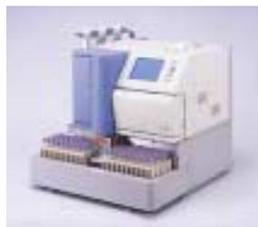
↑ Tosoh's ion-exchange HPLC is the gold standard for HbA1c measurement. The latest model of the Glycohemoglobin Analyzer is the HLC-723 G7.
