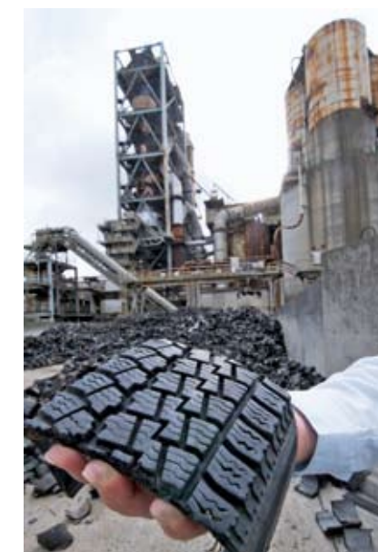
The cement plant at Tosoh's Nanyo Complex consumes scrap tires, plastic waste (below), and other difficult-to-dispose-of waste as fuel.
