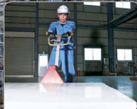
The electrolysis operations at Tosoh's Nanyo Complex yield an abundant supply of hydrogen, and the company uses some of that hydrogen to fuel high-temperature kilns for processing natural quartz into high-purity ingots.
