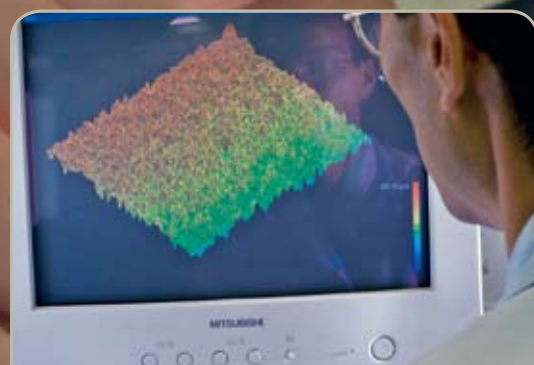
The monitor displays a microscopic textural rendering of the surface of an LCD coating under development at Tosoh.
