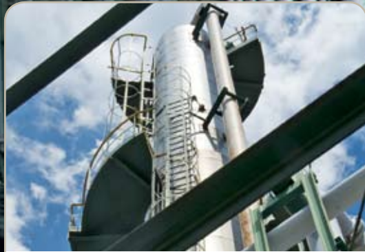
This plant at Tosoh's Yokkaichi Complex produces tertiary butyl alcohol to use in producing methyl methacrylate monomer.
